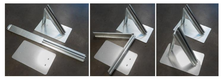
Ships Flat for quick assembly at worksite. #1: Bend the Upper Support Arm into a Triangle shape; #2: Insert the four corner tabs into the brackets; #3: Bend the corner tabs upward with **Pliers or Flathead Screwdriver**.
